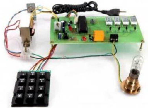
Figure 39: Programmable load shedding
